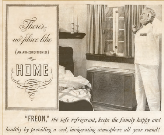
FIGURE 9 The chlorofluorocarbon FREON could be safely used in packaged air-conditioning equipment located in private or public places. (From: Kinetic Chemicals ad, Heating Piping and Air Conditioning , July 1934, p. 67).
